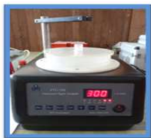
Figure 2 (c) Spin coating process
